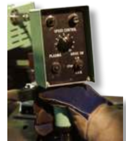
Remote Control Pendant allows safe control away from cutting workpiece
